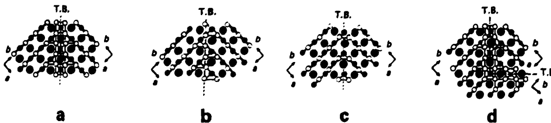
Fig. 29 - Idealized models of junction between twinning domains.
